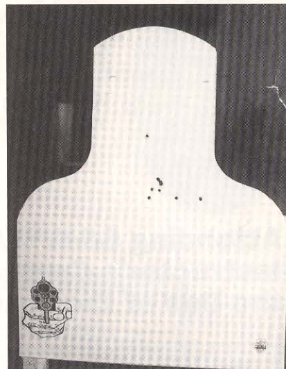
This 00 buckshot pattern was produced at 20 yards by an S&W Model 3000 pump set up with an 18-inch Vang Comp Systems modified barrel.
